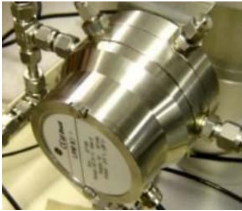
Fig. 10 Wet-wet differential pressure transducer assembly to enable connection between the cell pressure and back-pressure lines in the triaxial test. Note the pipe-work gives a “safe” position for initial set up whereby both sides of the central diaphragm of the transducer are connected to the same pressure giving a null or zero condition (permission of GDS Instruments).
