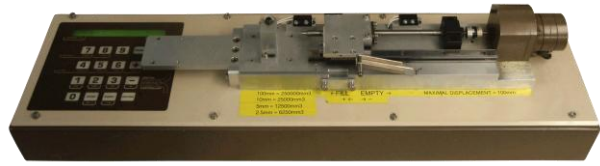
Fig. 7 Set-up of the rig used to calibrate Hall Effect transducers against displacement of a vernier micrometer. To avoid backlash the micrometer drum is turned in one direction (usually clockwise) during calibration.
