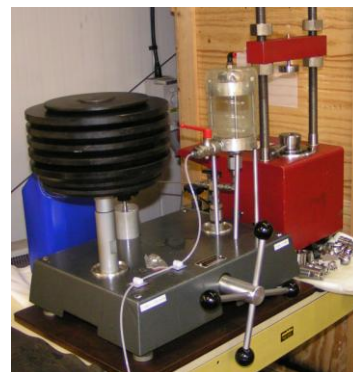
Fig. 3 Budenberg dead-weight tester showing stack of standard calibrating weights, oil-water change-over pot, and load cell calibrating frame (permission of DH-Budenberg Ltd).
