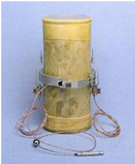
Fig. 5 One radial and two axial Hall Effect local strain transducers on a 100mm dia. Triaxial test specimen
