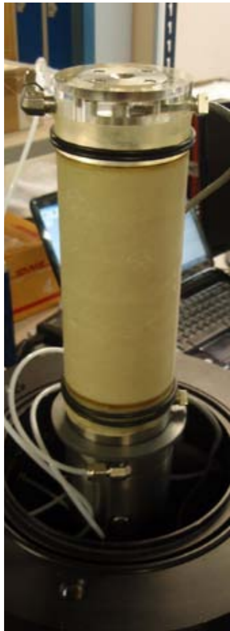
Figure 5 – Leighton Buzzard triaxial test specimen used to verify the performance of GDS BEAT (left); bender element signals obtained from the specimen (above).
