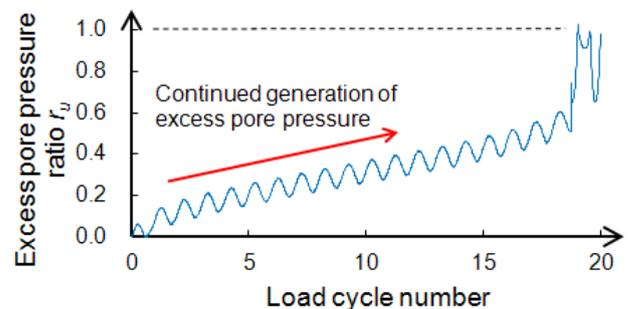
Figure 4 – Generation of excess pore water pressure during an undrained cyclic loading test on a sand specimen.
