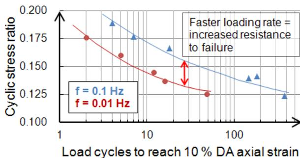
Figure 5 – Cyclic strength curves of Kaolin specimens for loading frequencies equal to 0.1 Hz and 0.01 Hz (data from Özyaydin and Erguvanli, 1980).
