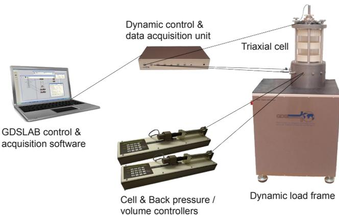
Figure 6 – GDS Dynamic Triaxial Testing System (DYNTTS) components.
