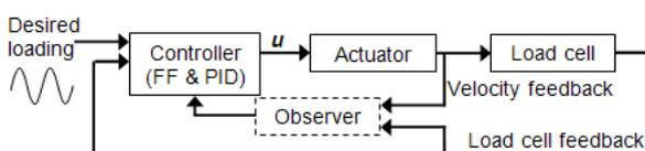
Figure 8 – New adaptive control method for GDS Dynamic Triaxial Testing System (DYNTTS).
