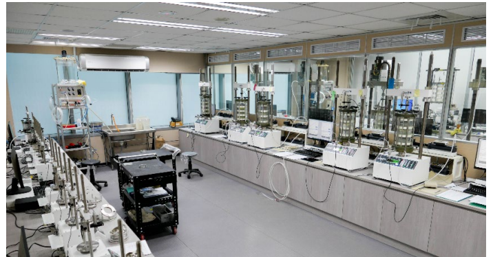
Photo taken showing the set-up of Triaxial Automated System (Right) and Oedometers (Left).
