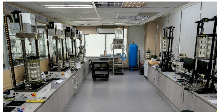
Photo taken showing the set-up of Enterprise Level Dynamic Triaxial Testing System (Left), Resonant Column Apparatus and Advanced Dynamic Triaxial Testing System (Right)
