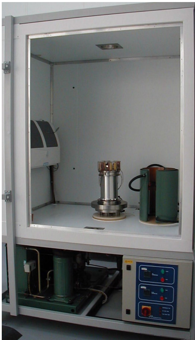
Fig 2. Southampton's RCA within its temperature control system. (Picture courtesy of University of Southampton)
