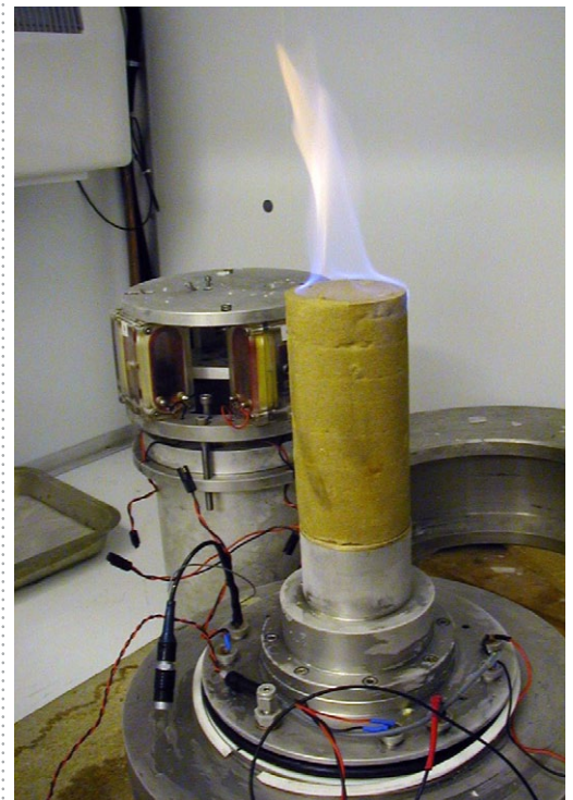
Fig 1. Methane burning as synthetic hydrate dissociates at the end of a laboratory stiffness test.
