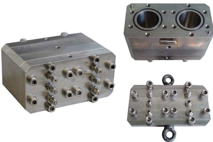
Fig 2. Shows CO<sub>2</sub> adsorption cell designed by GDS Instruments and Cardiff University
