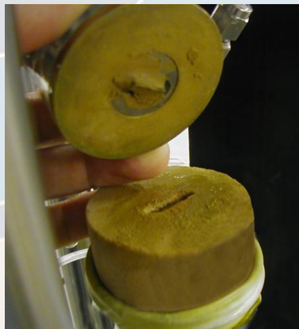
Fig 1. Shows the sandstone sample with the slot cut out for the bender element.
