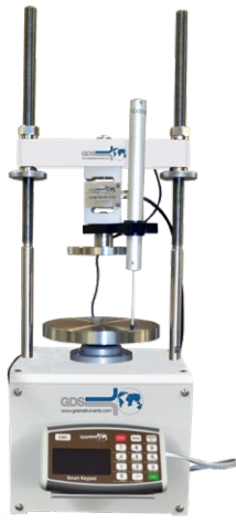
Unconfined Compressive Strength (UCS)
