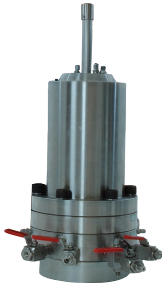
14MPa Triaxial Cell with 76mm max sample diameter (HP14/76)
