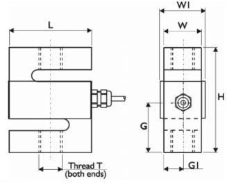
Note: On capacities over 100kN, cells will have rounded shoulders.
