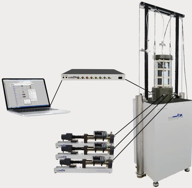
The GDS Hollow Cylinder Apparatus (GDSHCA) allows for rotational displacement and torque to be applied to a hollow cylindrical specimen of soil. Using this device it is possible to control the magnitude and direction of the three principal stresses. Studies can for example be made of the following:
