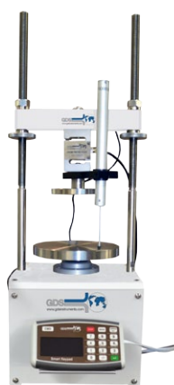
Unconfined Compressive Strength (UCS)
