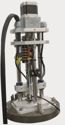
Actuator mounted onto cell (Covers removed)
