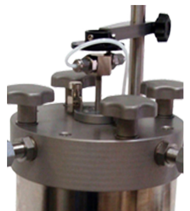
Fig. 3 GDS Rowe and Barden consolidation cell external axial displacement measurement point
