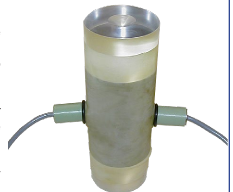
Fig 2. Horizontal elements mounted to specimen
