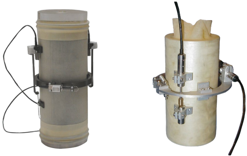
Fig. 11 Hall Effect and LVDT local strain transducers
