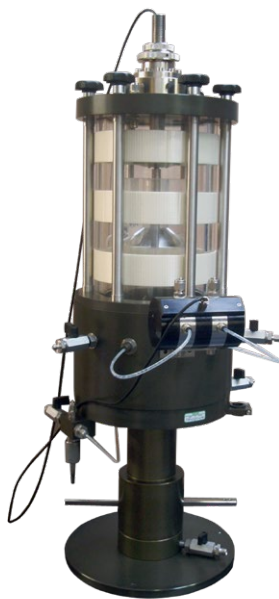
Fig 6a. Bishop & Wesley cell with cell top in place, inner cell and externally mounted Ultra low range DPT.
