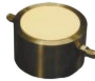
Fig. 1 HAEPD bonded into a standard triaxial pedestal
