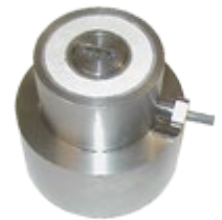
Fig. 2 HAEPD bonded into a bender element triaxial pedestal
