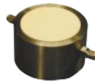
Fig. 1 HAEPD bonded into a standard triaxial pedestal
