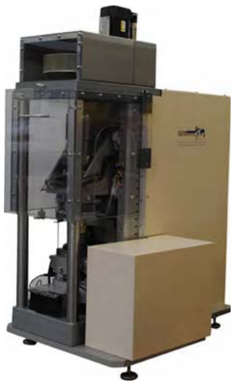
Figure 3 - The variable direction dynamic cyclic simple shear apparatus (VDDCSS), designed and built by GDS Instruments in cooperation with TUHH.
