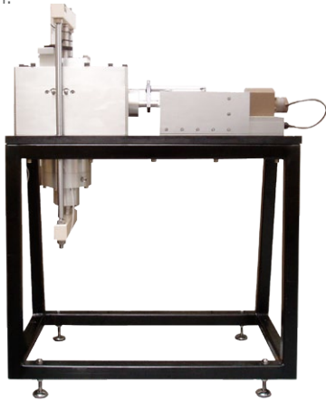
Figure 2: GDS Instruments Back Pressured Shear Box
