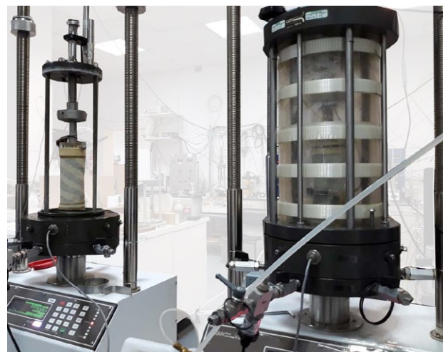
GDS Instruments hybrid cells in 50kN load frames at Geoteko laboratory in Poland.
