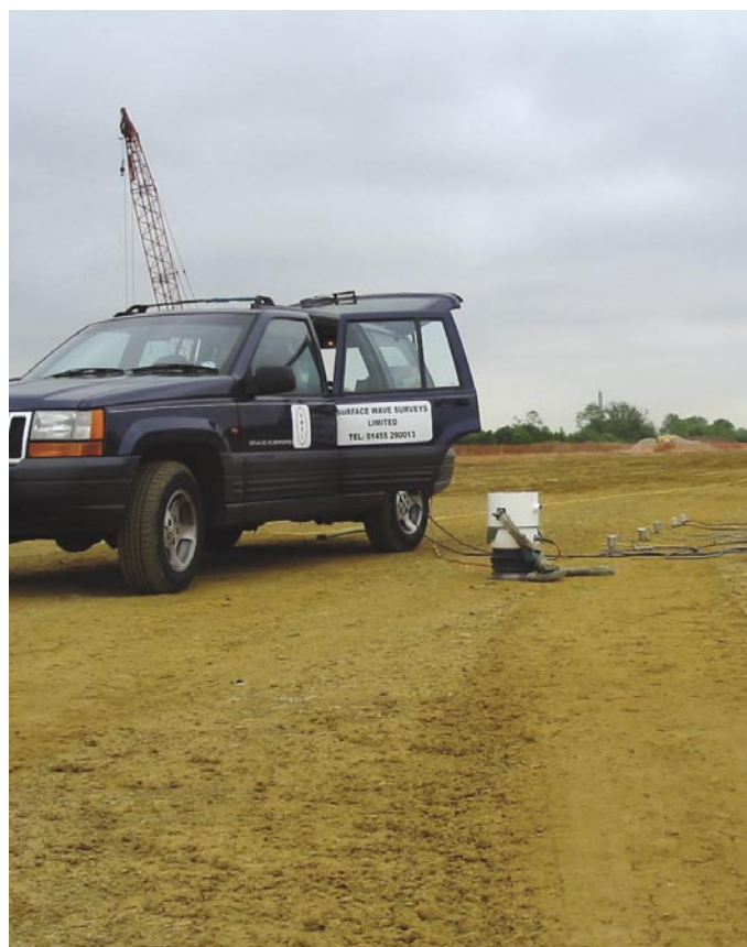
Figure 1: Continuous surface wave survey operation
