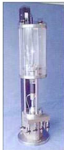
ABOVE: Figure 3. New motorised “stress path” triaxial cell.
