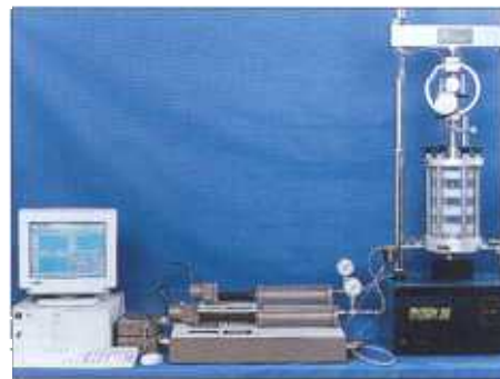
ABOVE: Figure 4. Triaxial Automated System for commercial labs.
