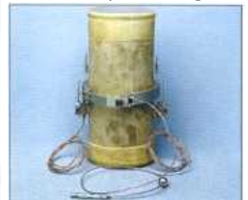
Figure 7. Triaxial test specimen with axial and radial Hall Effect local strain transducers.
