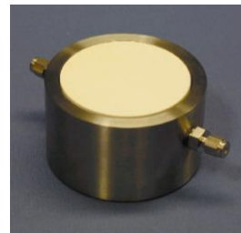
Fig. 1 HAEPD bonded into a standard triaxial pedestal
