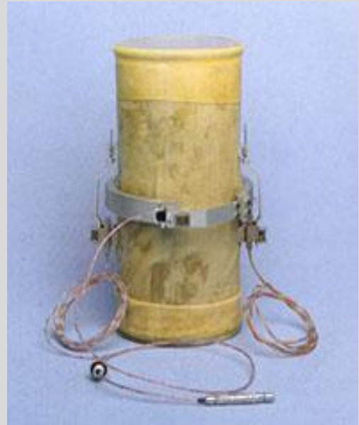
Fig 1: Radial and axial local strain transducers mounted directly on a triaxial test specimen
