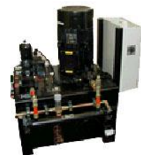
Fig. 2 GDS Hydraulic Power Unit
