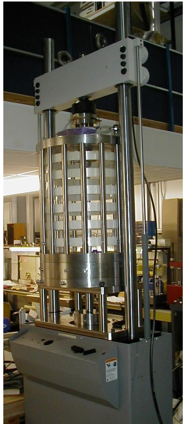
Fig. 1 LDCTTS testing system at the GDS factory
