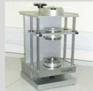
Fig. 7 HCA soil lathe
