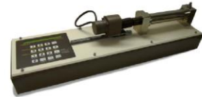
GDS Advanced Pressure/Volume controller, range from 100kPa to 150,000kPa
