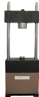
GDS axial loading Frame, range from 10kN to 500kN
