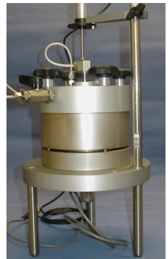
Fig. 4 GDS Rowe and Barden consolidation cell
