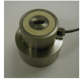
Fig. 4 HAEPD bonded into a bender element triaxial pedestal
