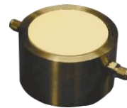
Fig. 4 HAEPD bonded into a standard triaxial pedestal
