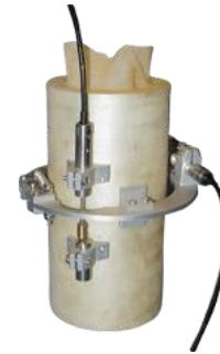
Fig. 3 Hall Effect and LVDT local strain transducers
