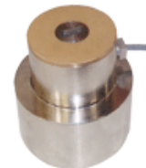
Fig. 5 HAEPD bonded into a bender element triaxial pedestal
