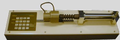
Fig. 2 2MPa/1000cc air pressure/volume controller
