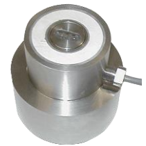
Fig. 4 HAEPD bonded into a bender element triaxial pedestal
