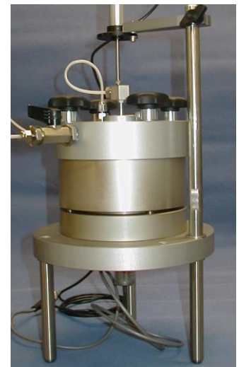
Fig. 4 GDS Rowe and Barden consolidation cell
