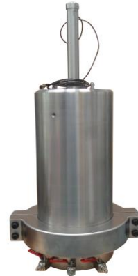
Fig. 8, 14MPa Triaxial Cell with 300mm sample height
