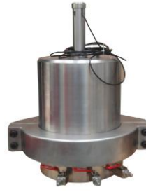
Fig. 7, 14MPa Triaxial Cell with 80mm sample height
