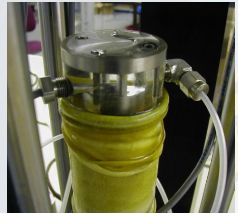
Fig 2. Shows the bender element sample within the triaxial cell.
